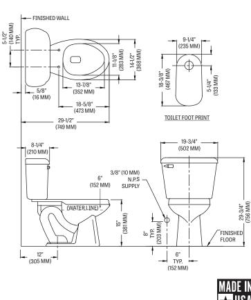
Fixture performance and specifications meet or exceed ASME A112.19.2/CSA B45.1 standards, and other state and local codes.
